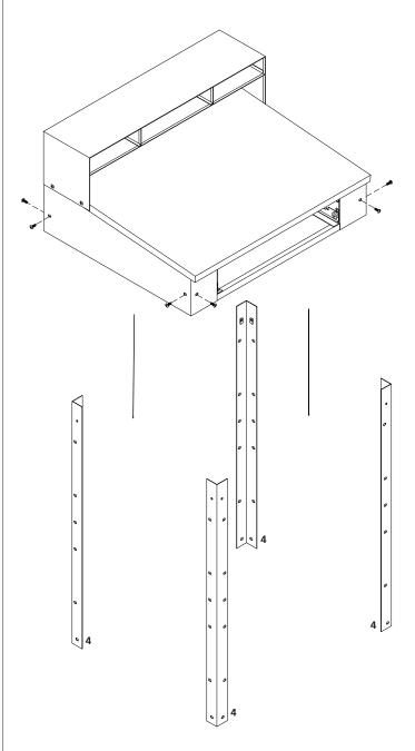
**3.** Attach the shelf supports (Ref. No. 3) to the front legs, using one bolt on each leg. Next, place the shelf (Ref. No. 5) into position and bolt the shelf and shelf support to the rear legs, again using one bolt per leg. Secure the shelf by bolting it to each shelf support.
